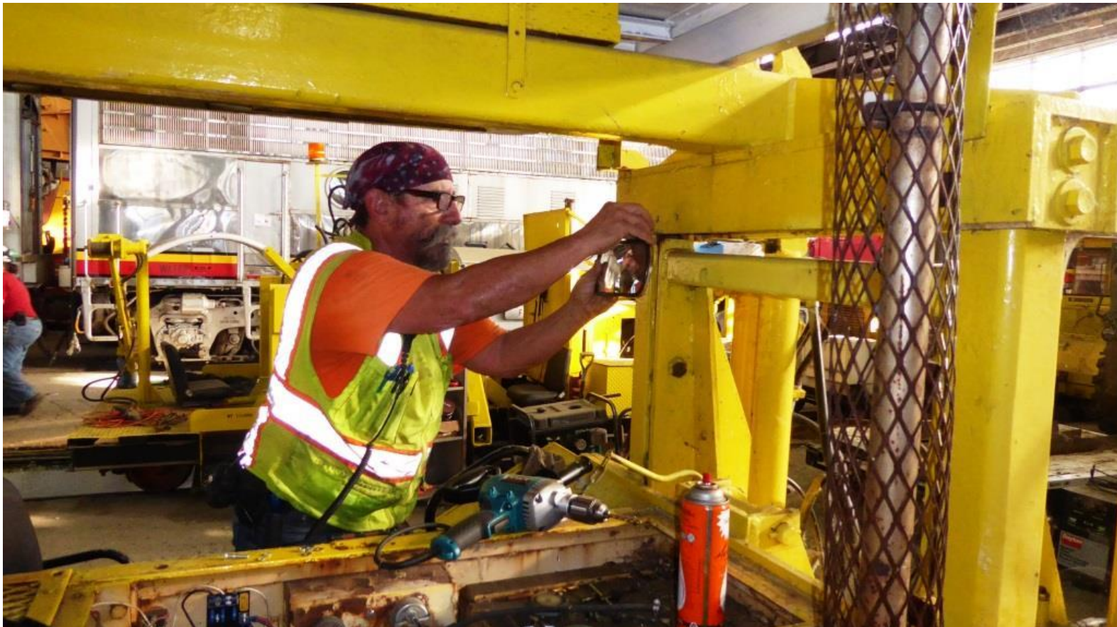
Joe installs a rear-view mirror on the Jackson 125 tie-exchanger
